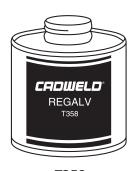
T358 Regalv is a 97% zinc rich organic coating which also can be used to repair galvanized surfaces. The brush is attached to the cap.
